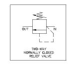
Relief valves (Pressure Safety Valves) are designed or set to open at a predetermined set pressure to protect other equipment from being subjected to pressures that exceed their design limits.
