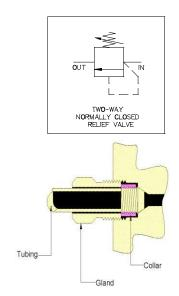
Medium pressure tubing, tubing size is 1/4" ODX0.109"ID, 1/4"Medium Pressure (LF4)]
