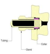
Medium pressure tubing, tubing size is 1/4" ODX0.109"ID, 1/4" Medium Pressure(LF4)
