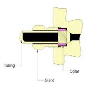
Medium pressure tubing, tubing size is 1/4" ODX0.109"ID, 1/4" Medium Pressure(LF4)
