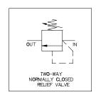
Relief valves (Pressure Safety Valves) are designed or set to open at a predetermined set pressure to protect other equipment from being subjected to pressures that exceed their design limits.
