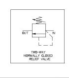
Relief values (Pressure Safety Values) are designed or set to open at a predetermined set pressure to protect other equipment from being subjected to pressures that exceed their design limits.
