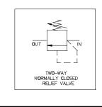
Relief valves (Pressure Safety Valves) are designed or set to open at a predetermined set pressure to protect other equipment from being subjected to pressures that exceed their design limits.
